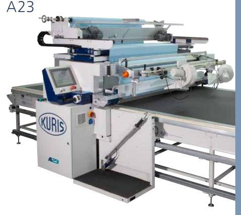
The A23 is an innovative spreading machine which is also very suitable for critical, smooth and elastic fabrics or poorly wound rolls of material. Strain-sensitive goods are spread without any tension. In the 1920s, fabrics were hung up precisely in multiple layers on what were known as rectometers from our company, tilted and supplied for precision cutting. Today the materials are spread out directly from the roll.
