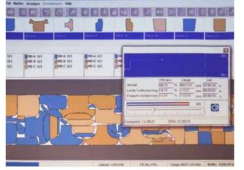
Computer Aided Design. What this means for cutting technical textiles and all kinds of other textiles is: How does the required cutting shape get to the cutting machine as quickly as possible? This on its own is a broad topic. Whereas previously a pantograph was able to transfer a contour from the original to the copy, nowadays the contours can be recorded with a digital photo of a pattern and reconstructed as many times as you want.
