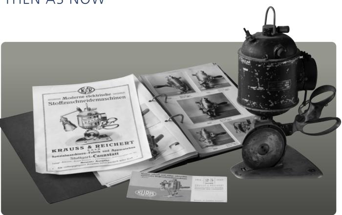
The history of Kuris began with the electrical handheld cutting machines. The first models still had grips like scissors to make it easier for users to make the switch. Quite a lot has changed since then, but the range of applications has remained the same. Handheld machines are employed wherever any kind of fabric needs
