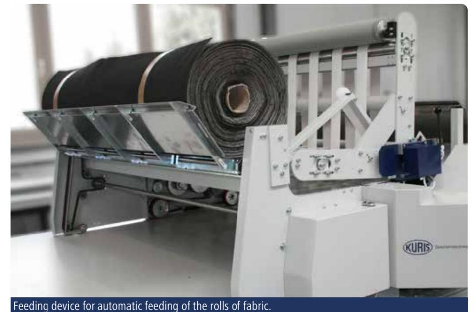
Feeding device for automatic feeding of the rolls of fabric.
