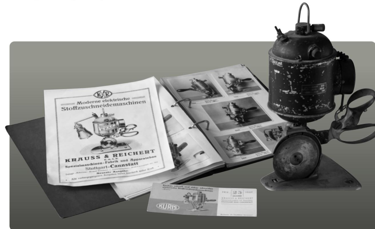
The history of Kuris began with the electrical handheld cutting machines. The first models still had grips like scissors to make it easier for users to make the switch. Quite a lot has changed since then, but the range of applications has remained the same. Handheld machines are employed wherever any kind of fabric needs to be cut in small quantities or with varying contours. Today they are of course also available as a battery-powered version.
