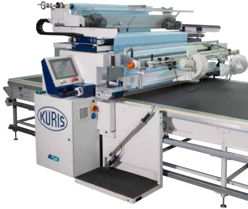
The A23 is an innovative spreading machine which is also very suitable for critical, smooth and elastic fabrics or poorly wound rolls of material. Strain-sensitive goods are spread without any tension. In the 1920s, fabrics were hung up precisely in multiple layers on what were known as rectometers from our company, tilted and supplied for precision cutting. Today the materials are spread out directly from the roll.
