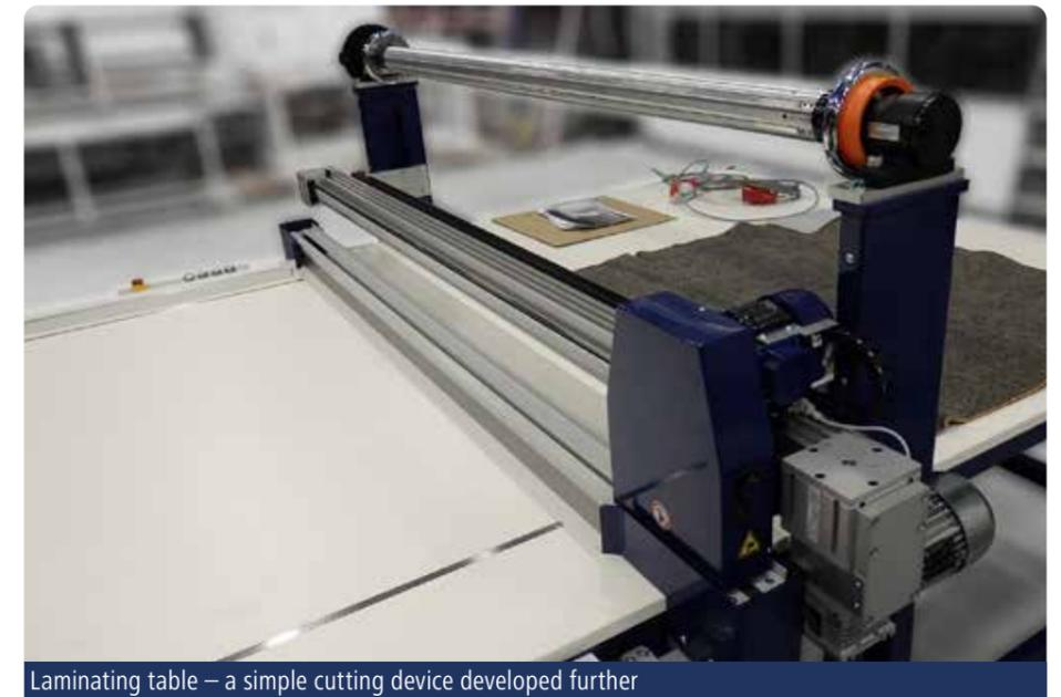
Laminating table – a simple cutting device developed further
