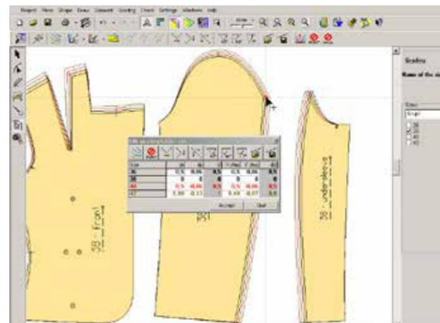
Computer Aided Design. What this means for cutting technical textiles and all kinds of other textiles is: How does the required cutting shape get to the cutting machine as quickly as possible? This on its own is a broad topic. Whereas previously a pantograph was able to transfer a contour from the original to the copy, nowadays the contours can be recorded with a digital photo of a pattern and reconstructed as many times as you want.
