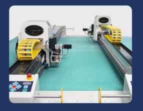
Optionally with double bridge: Two bridges for independent cutting with two cutting heads in one cut pattern. Cutting time saving: up to 40%
